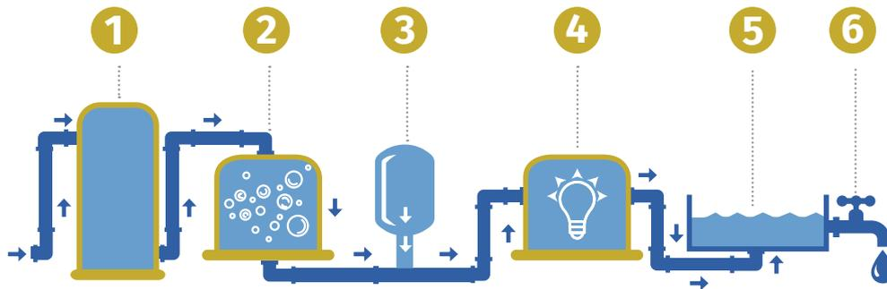
**1** Granular Activated Carbon Filled (GAC) Vessels remove VOCs to below detection levels.
